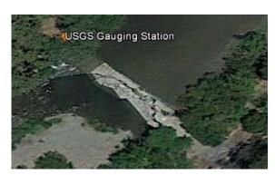
This failing cement apron is part of a gauging station used to measure stream flow in Alameda Creek. It is impassable to steelhead trout and other native fish at low flows. A new gauging station is in place, but continued use of this gauge allows scientists to properly calibrate the new data with historic.
